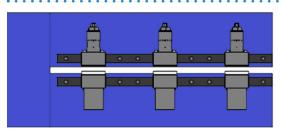
This HOLE PNEUMATIC PUNCHING MACHINE is a device that occupies little space and is designed to punch holes in the OUTER EDGE OF THE MOVING FILM and in particular, it works with PLAIN OR PRINTED FILM. This PU model has to be integrated into EXISTING
